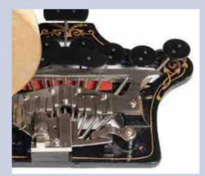
A view from the back shows the Stenograph's key arms -- v-shaped connected bars. With these connections, the manufacturer considered the Stenograph to be a five-keyed machine.
