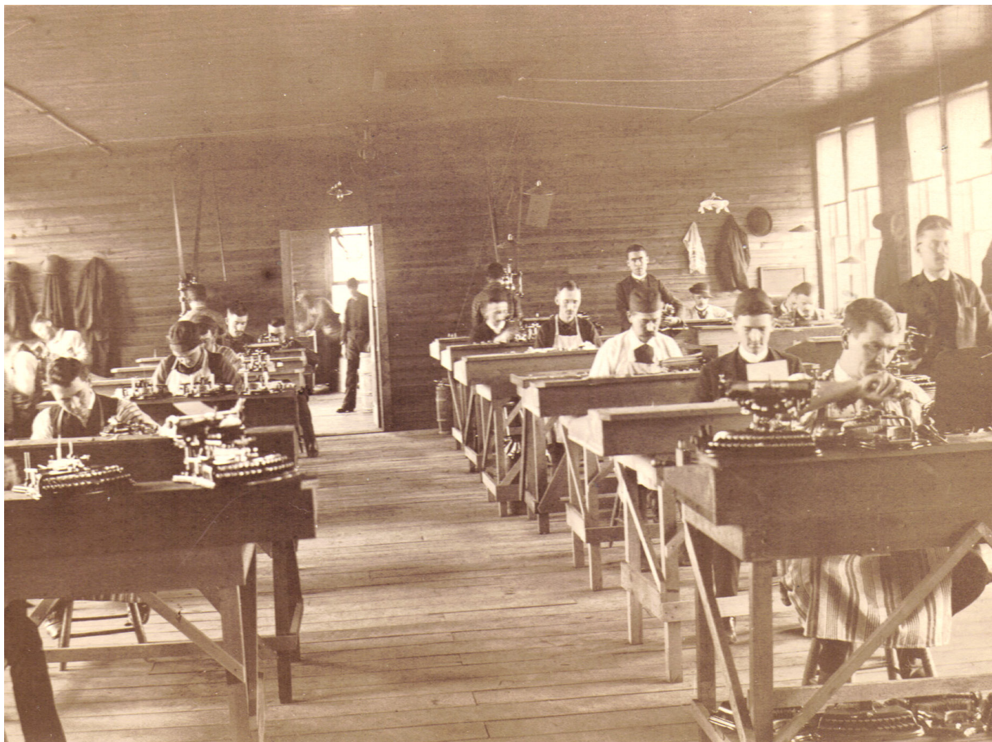
This exceptional photograph (Clark Coll.) shows the interior of the Crandall typewriter Co. in Groton, N.Y., during the first half of 1887, when Crandall 1 typewriters were made exclusively there. Twenty-two typewriters can be seen in the photo in various states of assembly.
