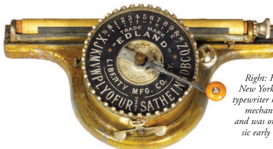
Edland - New York - 1892: To type on this intriguing typewriter, one moves the index pointer around to a character and then pushes down. Under the index plate is a daisy wheel, with each character on a flexible brass 'finger', which is pushed to the paper to print.
